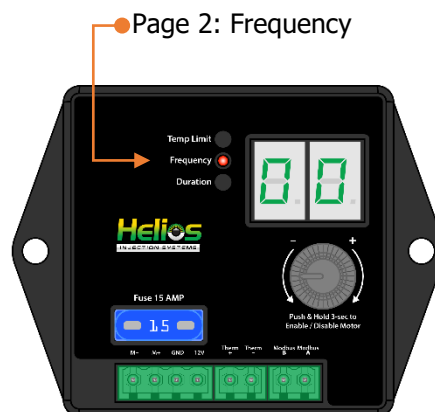
How many times the motor turns on per minute. Values can be set between 0-10
