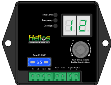
No "Page" LED on showing Battery Voltage: 12V
